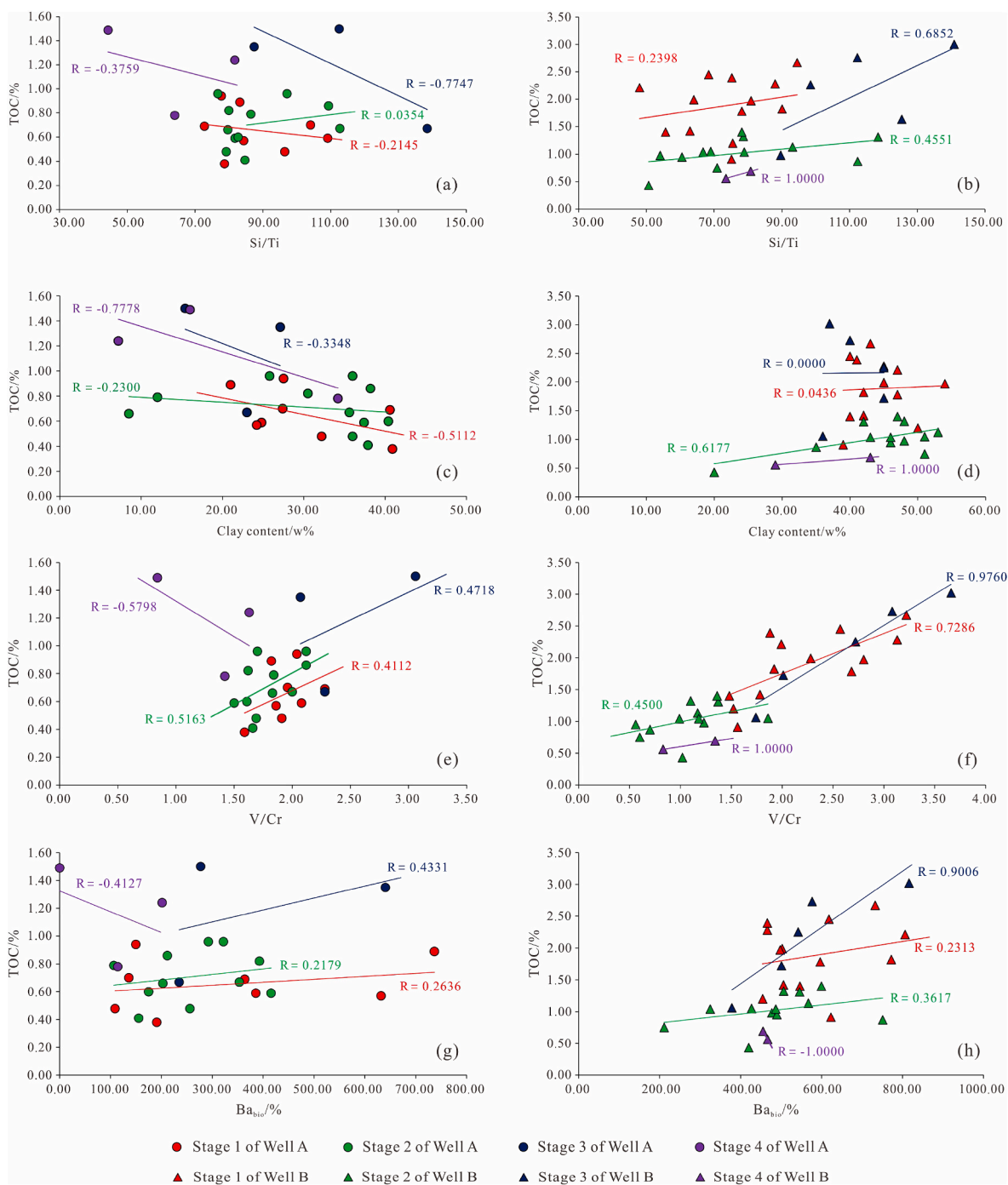
Fig. 12. Cross plots of Si/Ti of Well A (a), Si/Ti of Well B (b), Clay content of Well A (c), Clay content of Well B (d), V/Cr of Well A (e), V/Cr of Well B (f), Ba bio of Well A (g) and Ba bio of Well B (h) versus TOC.
